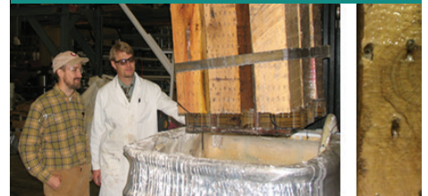
Adam Taylor, left, and Jeff Lloyd of Nisus perform original ambient temperature borate treatments.
